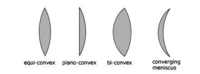
All four types of convex lens are converging lenses. That is, they bring parallel rays of light to a focus, producing a real image.
