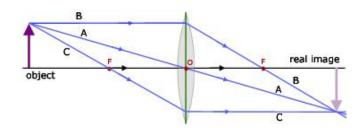
A) a ray passing through the optical centre of the lens
