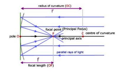
The basic ray diagram for a concave mirror introduces a number of important terms: **aperture** - the diameter of the circular mirror **pole** - where the principal axis meets the mirror surface **centre of curvature** - the centre of the sphere that the mirror forms part **radius of curvature** (r) - radius of the sphere **principal axis** - the line through the centre of curvature and the pole of the mirror **focal length** (f) - equal to half the radius of curvature f = r/2<u>Ray Diagrams</u>
