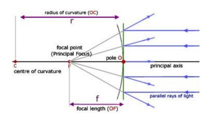
The basic ray diagram for a convex mirror introduces a number of important terms:
