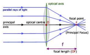
The basic ray diagram for a convex lens introduces a number of important terms:
