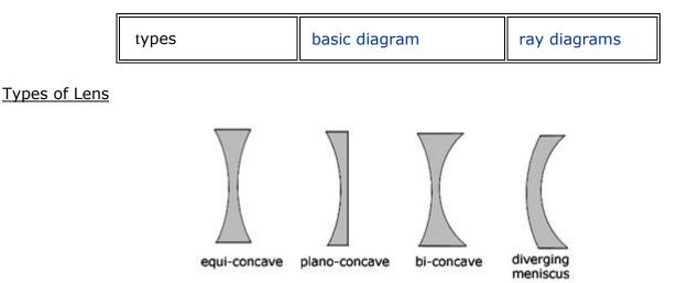
All four types of concave lens are diverging lenses. That is, they diverge parallel rays of light from a focus, producing a virtual image.
