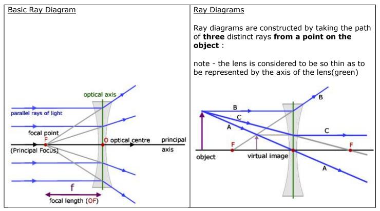
**A**) a ray passing through the optical centre of the lens
