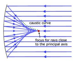
The **caustic** is the name given to the region of a concave mirror where parallel rays of light come to different foci.
