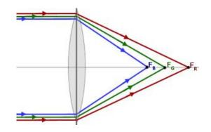
Chromatic aberration affects the image by making it appear blurred with fringes of colour around it. This is a result of only one colour being in focus at a time.
