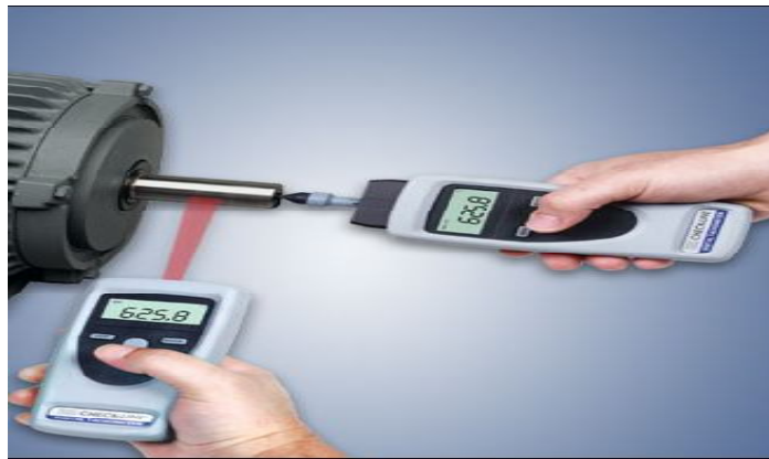
Fig. 5.6 Use of Digital Tachometer
