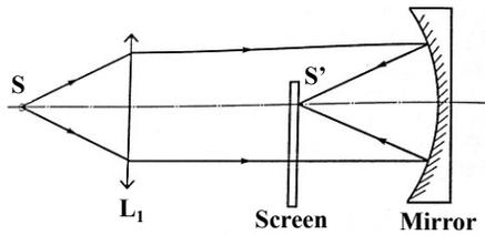
Figure 3: Measurement of the focal length of a concave mirror
