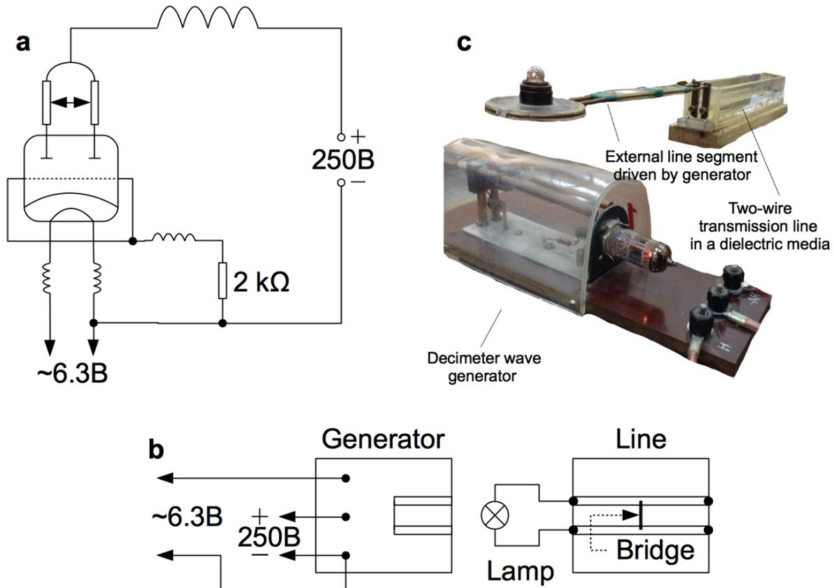
Figure 1: Experimental setup: a) biasing scheme of the lamp decimeter wave generator; b) position scheme of the elements of the setup; c) photos of actual elements of the setup.
