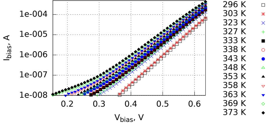
**Figure 5.** IV curve as a function of the diode's operating temperature. Y-axis is given in the logarithmic scale.
