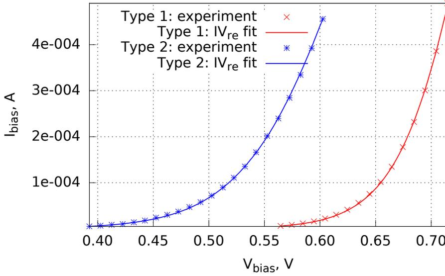
**Figure 7.** The IV curve of the PSD sample measured at ambient temperature.
