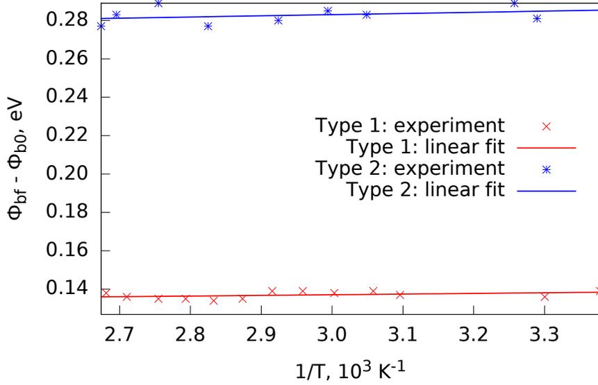
**Figure 6.** The difference of the flat band and the zero bias current barrier heights as a function of the inverted operating temperature of the PSD sample.
