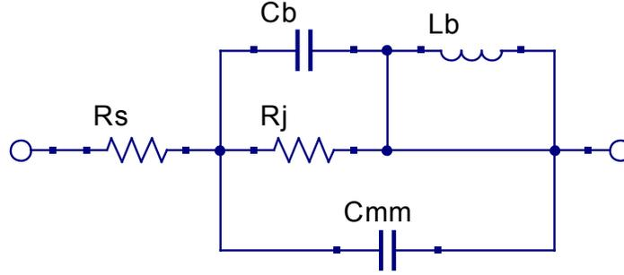
**Figure 4.** The lumped element model of the inner part of the PSD sample. Here  $R_s$  is the series resistance,  $R_j$  is the junction resistance,  $L_b$  is the inductance of the suspension bridge,  $C_b$  and  $C_{mm}$  are the 'bridge-to-mesas' and 'mesa-to-mesa' capacitances, respectively
