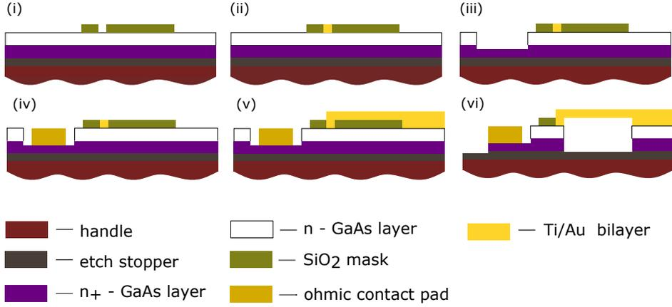
**Figure 1.** Main stages of the PSD fabrication process.
