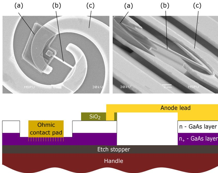
**Figure 2.** SEM images containing top (top panel, left) and side (top panel, right) views of a quasioptical PSD, and a schematic of its layered structure (bottom panel). Here (a), (b) and (c) denote the ohmic contact pad, the anode lead and the antenna arm, respectively.
