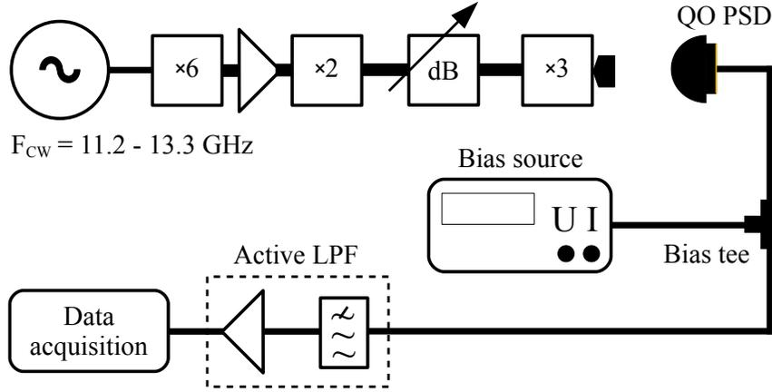
Figure 3. Experimental setup.
