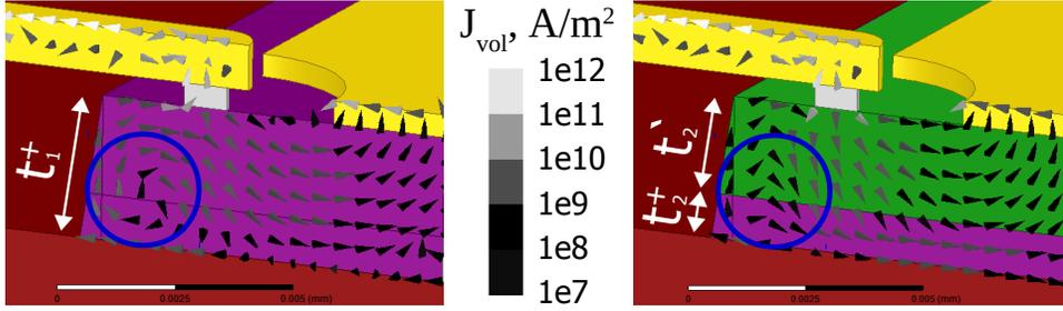
**Figure 9.** The calculated current density distribution within the layered structure of a PSD of type 1 (left) and type 2 (right) at 450 GHz. The coloring is identical to that provided in figure 1 except for the additional 'green' layer denoting the n'-GaAs matching sublayer.
