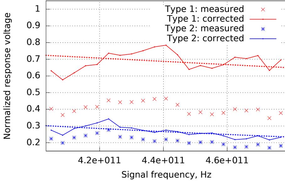
**Figure 8.** Response voltages of the quasioptical PSD samples as a function of the signal source's frequency. The dotted lines denote the corresponding RC fits.
