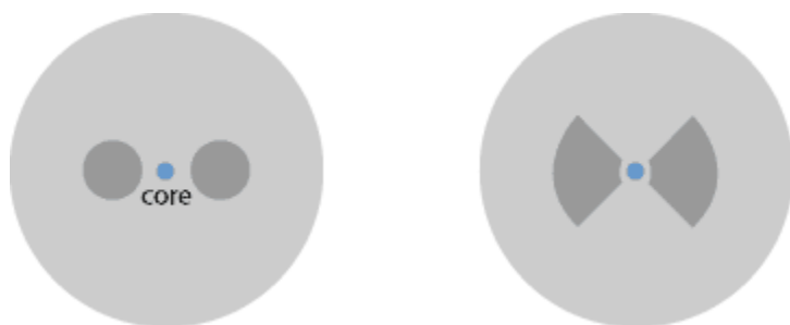
Figure 2: Polarization-maintaining PANDA fiber (left) and bow-tie fiber (right). The built-in stress elements, made from a different type of glass, are shown with a darker gray tone.
